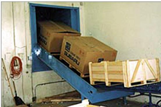
A system was designed around a **low-speed BloApCo vertical pallet shredder** with patented "**Pierce-and-Tear**" action that substantially reduces noise, dust and throw-out of shredded pieces. Complete crates and pallet bins (as large as 58" wide by 48" high) are loaded onto a 60" wide infeed conveyor inside the building which transports the material through a wall opening, discharging directly into the shredder. The shredded pieces then drop into a compactor.
