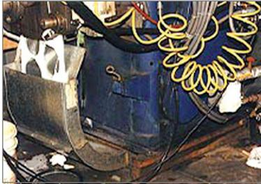
**Altra Filters, Inc.**, is the largest producer of coffee filters in the U.S., with plants on the east and west coasts. In the Riverdale, NJ, plant, the company operated five punch presses, each producing 50 filters per stroke. The filter paper was fed to the presses from 50 rolls mounted on backstands at about 60 strokes a minute, in a horizontal plane, so the continuous web of paper waste (matrix) fell downward as the press retracted.
