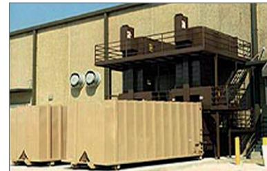
Shredding before compacting increases the amount of material that a 40 cu. yd. container can hold – from only 8,000 pounds of cartons (compacted only) to an efficient 18,000 to 20,000 pounds of shredded, compacted material. They now only have three containers that are hauled away versus their prior need of hauling seven containers that were filled with non-shredded material.
