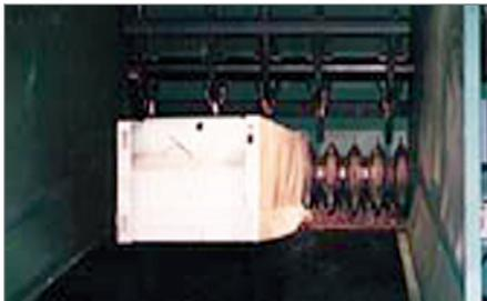
**A 48" top-feed BloApCo "Pierce-and-Tear" shredder,** specifically configured to handle the bulky irregularly shaped liners, was installed above the granulator. The shredder reduces the liners into pieces that can be readily and easily ingested by the granulator.
