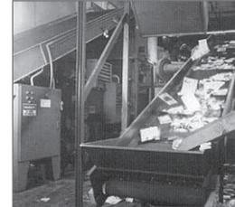
They found that when they were feeding at maximum volume, some magazines were not being thoroughly shredded, and the shredder was having trouble keeping up. Bale quality was poor. In addition, they also needed to shred corrugated and newspapers which require a slightly different shredder than one for books and magazines.
