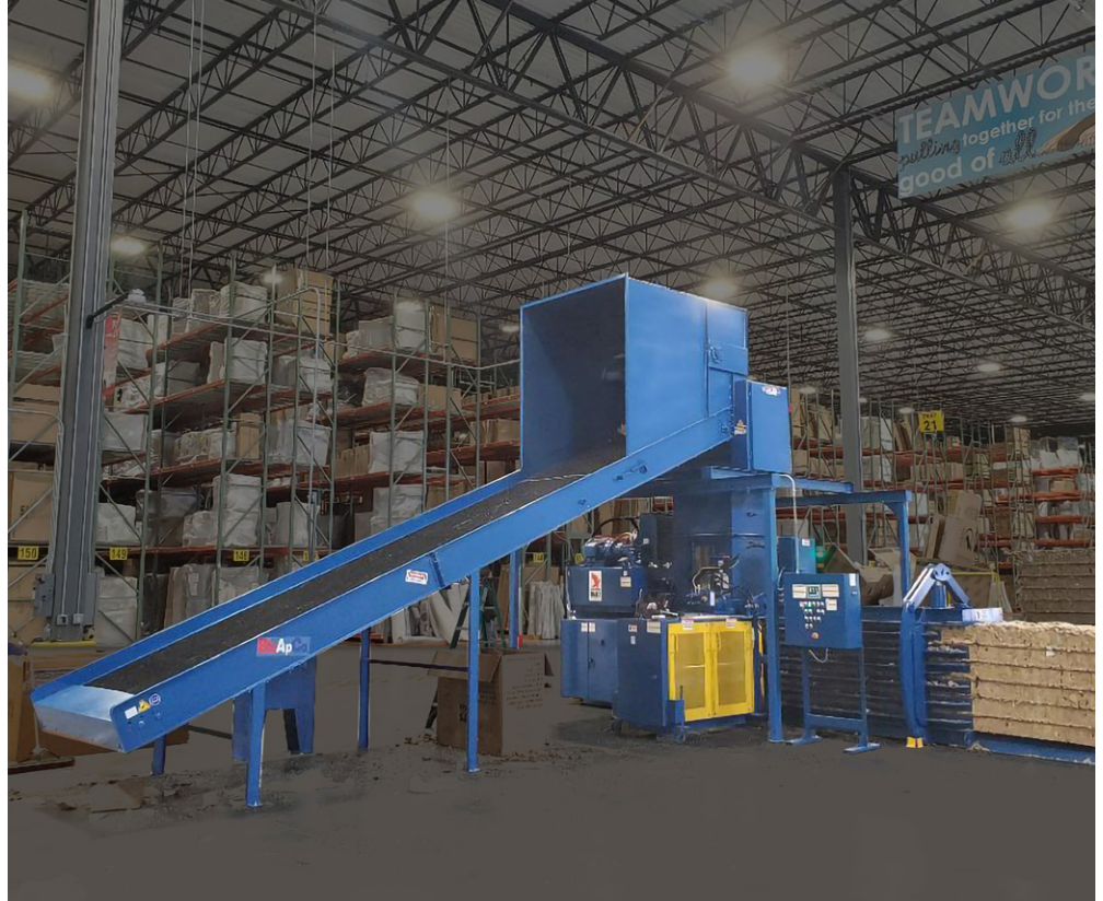
A BloApCo piggyback shredder with a box crusher mounted over a horizontal auto-tie baler.
